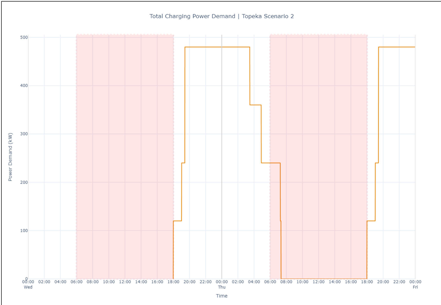
Figure 44. Scenario 2: Midday Charging in Depot and at QSS (Short Top-Ups) – Overnight Charging Power Demand (Wednesday-Thursday Shown)
