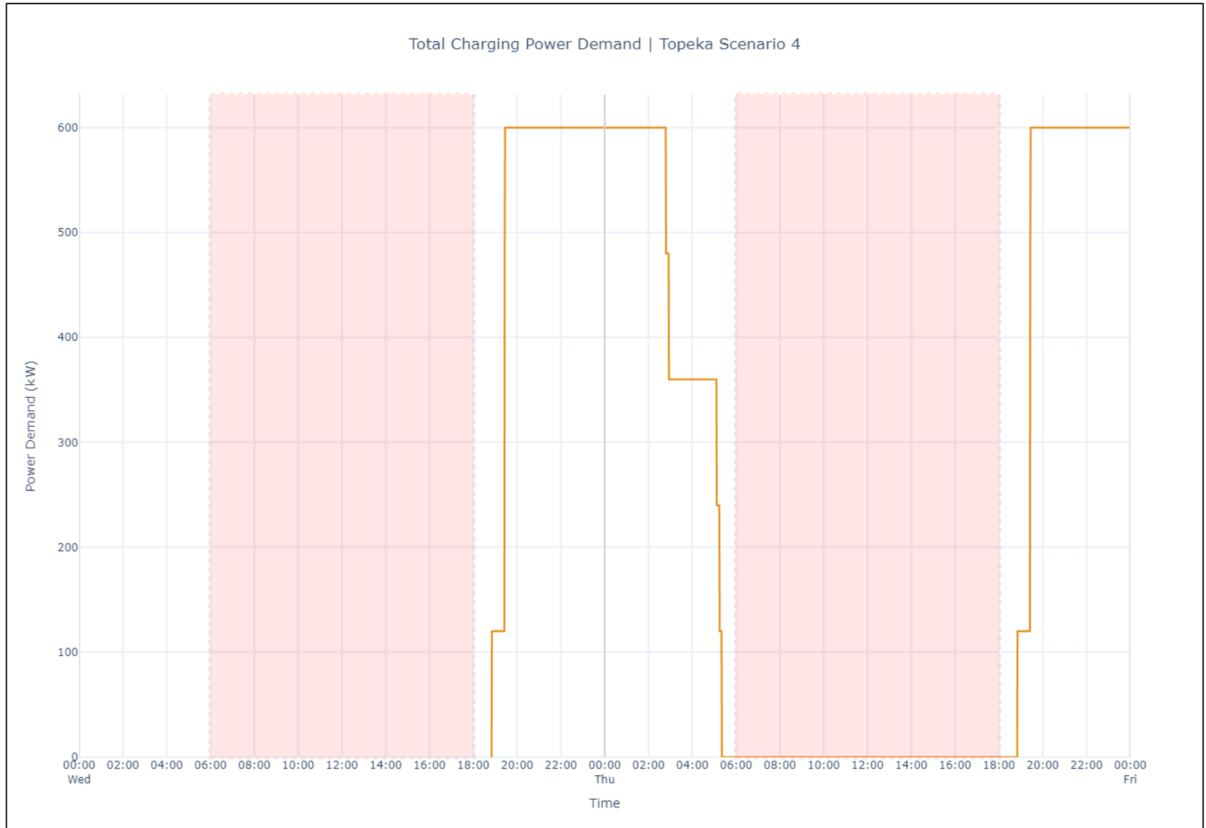
Figure 60. Scenario 4: Midday Charging in Depot Only, Enlarged Battery Size – Overnight Charging Power Demand (Wednesday-Thursday Shown)
